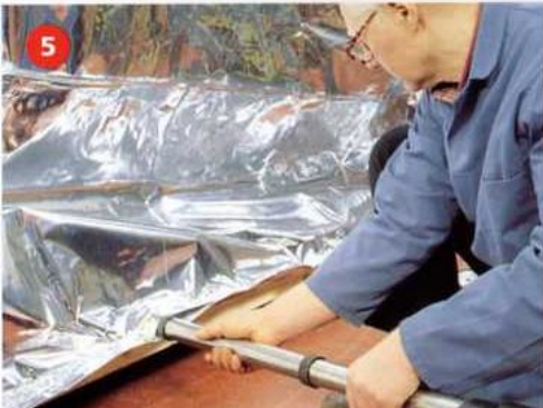
5 Foil bag is lined up with base sheet. Excess air is removed.
